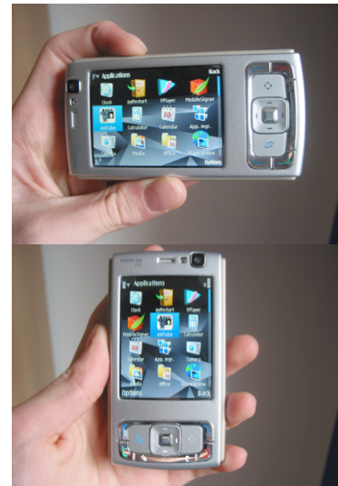
Figure 1: Some of today's cell phones use accelerometers that allow you to turn the phone on its side and still produce the same picture
